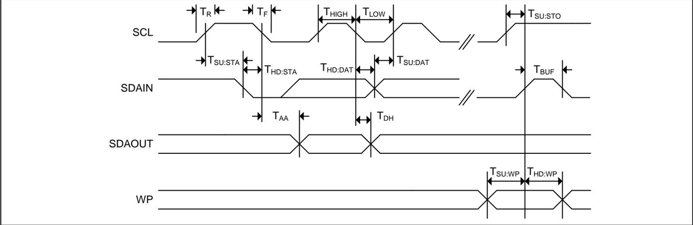
Figure 5-12. Write Cycle Timing
